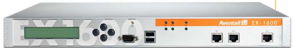
The EX-1600 detects the identity and security state of remote devices, protects against unauthorized access by enforcing granular policy and connects users seamlessly to mission-critical enterprise resources.
